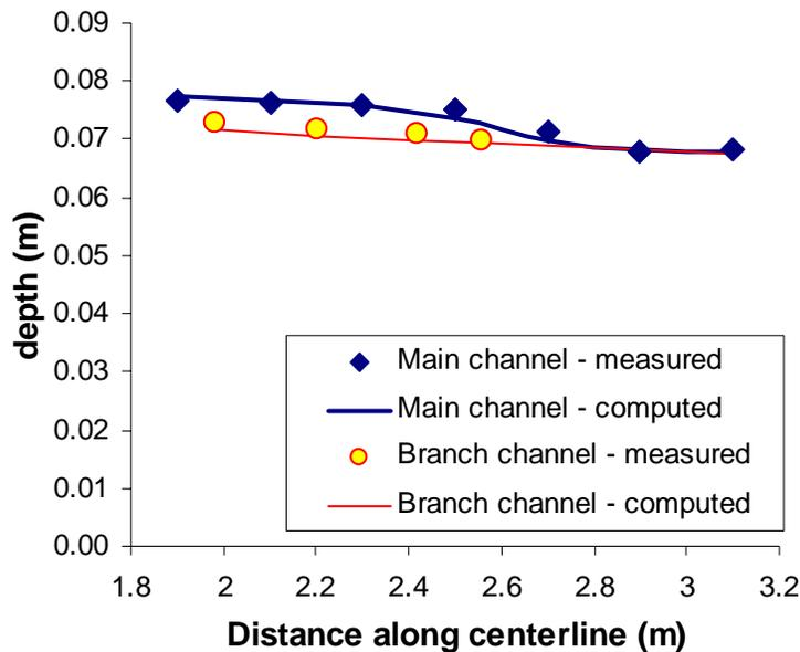
Figure 3. Measured and computed longitudinal water depth profiles along main and branch channels for  $30^\circ$  diversion (Bulle 1926).
