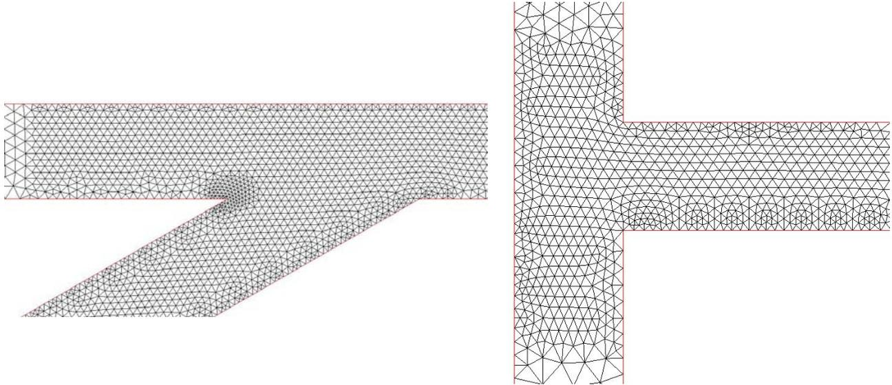
Figure 1. Details of the Finite Element mesh around the entrance to the branch channel for Bulle's 30° diversion (left plot) and Barkdoll et al.'s 90° diversion (right plot).
