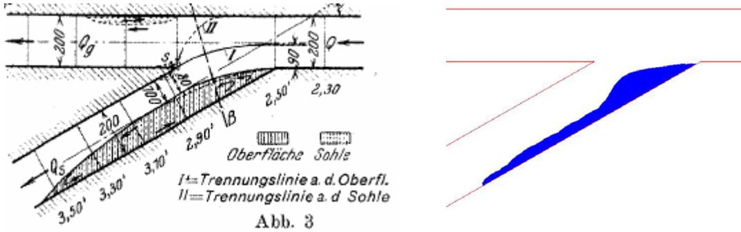
Figure 2. Extension of the recirculation zone in the diversion channel measured by Bulle (left plot) and predicted by River2D (right plot).
