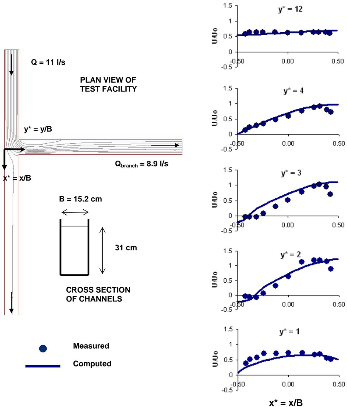
Figure 6. Layout of Barkdoll et al. (1998) test facility and experimental conditions, showing also the computed streamlines and a comparison between measured and computed velocity profiles along the branch channel.
