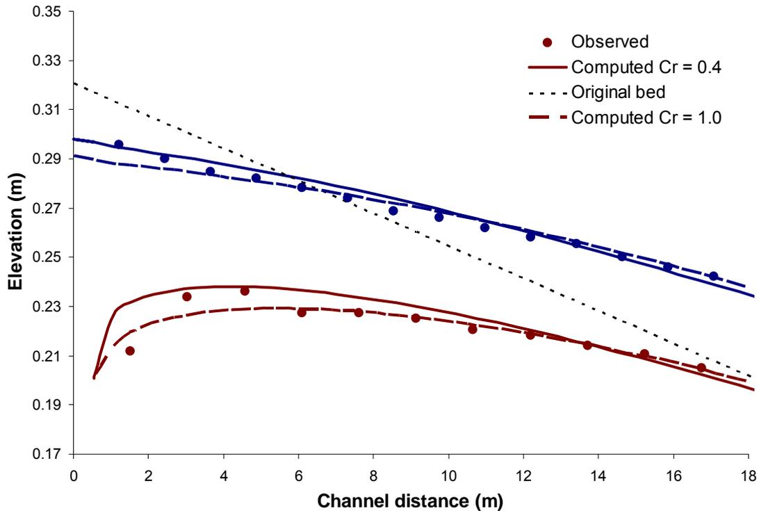
Figure 3. Observed and computed longitudinal profiles at 10 hours for bed degradation experiment due to sediment supply shut-off for two correction coefficient values  $C_r = 1.0$  and  $C_r = 0.4$ .
