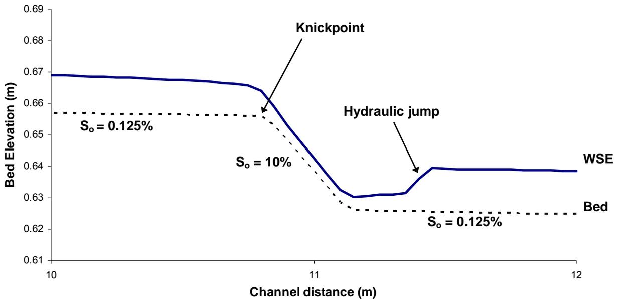
Figure 4. Initial conditions for knickpoint migration experiment ( $t = 0$ ). Water surface elevation was computed by the numerical model.
