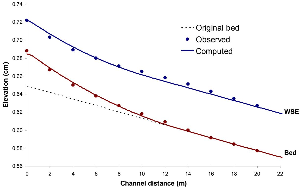
Figure 1. Observed and computed longitudinal profiles at 40 minutes for bed aggradation experiment due to an overload of sediment equal to four times the equilibrium value.
