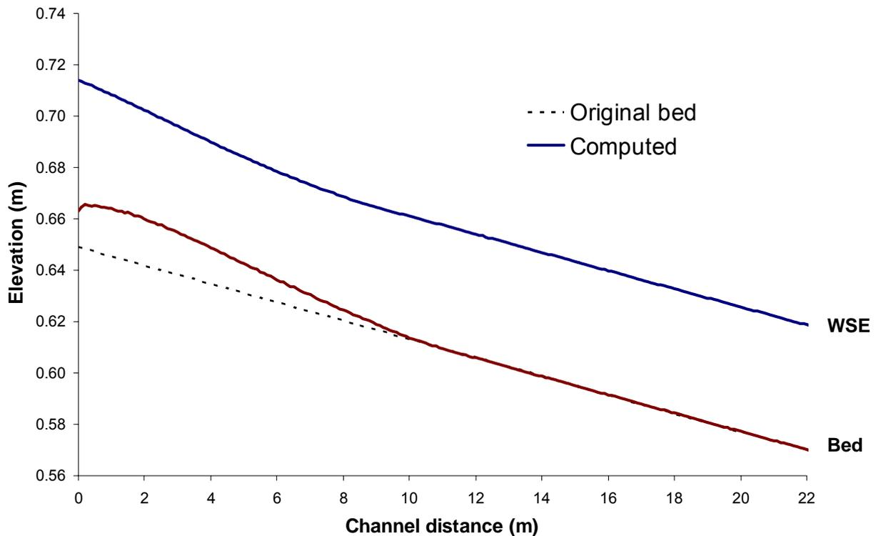
Figure 2. Computed aggradation profiles at 40 minutes with unsteady inflow of sediment as upstream boundary condition.
