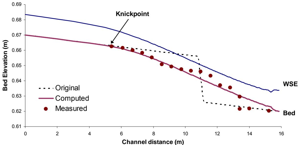
Figure 5. Observed and computed longitudinal profiles at  $t = 2 \text{ hr } 40 \text{ min}$  for knickpoint migration experiment.
