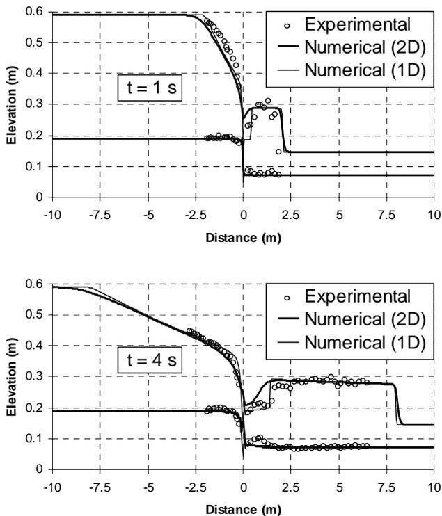
Figure 8. Experimental and numerical results for dam-break experiment Ts.28 at 1 and 4 seconds.
