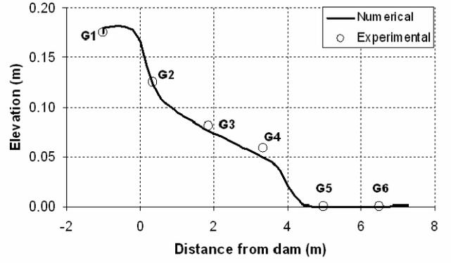
Figure 2. Experimental and numerical results at 2.5 s for dam break through a 90° bend.
