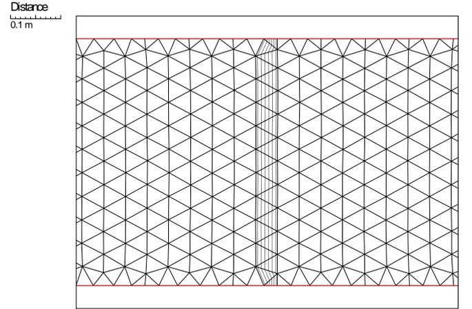
Figure 6. Detail of unstructured mesh near the dam location (dashed lines are bed contours of inclined ramp).
