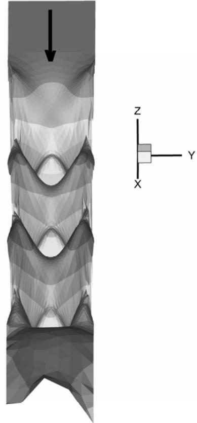
Figure 4. 3D view of computed bed changes in a channel with sinusoidal varying width.
