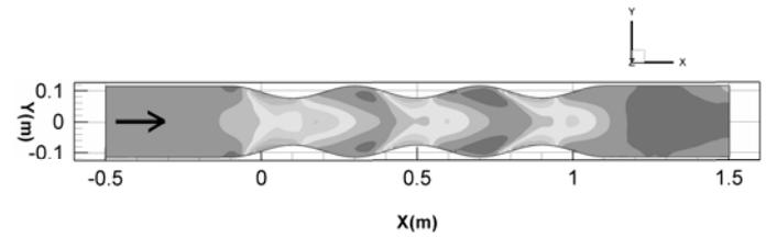
Figure 3. Plan view of computed bed changes in a channel with sinusoidal varying width.
