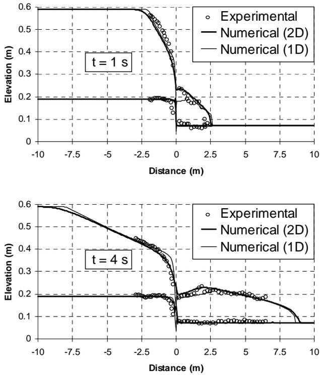
Figure 7. Experimental and numerical results for dam-break experiment Ts.25 at 1 and 4 seconds.
