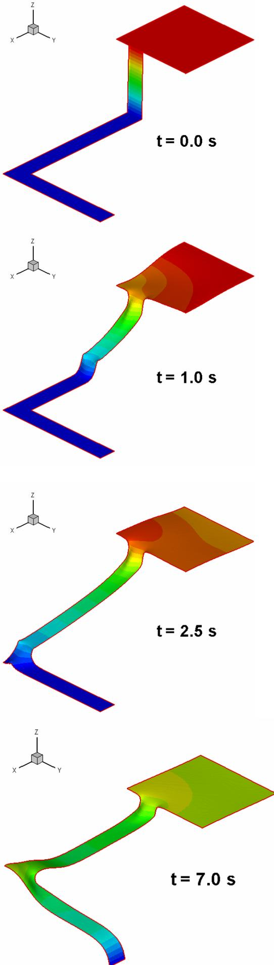
Figure 1. Computed water surfaces for a dam-break in a channel with a 90° sharp bend.
